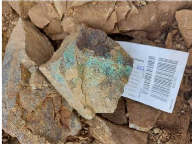
Altered and veined granodiorite from the Mint - assays returned 0.17% Cu and 1.37 g/t Au
