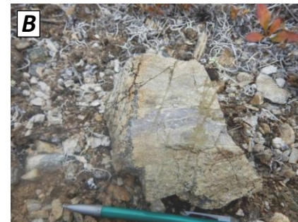
A) Quartz-biotite-magnetite veins developed within k-feldspar altered porphyry from the core zone of the Maloney area; B) Thin epidote-chlorite veins overprinting quartz-sericite veins within a strongly altered, quartz-sericite-pyrite porphyry from the Maloney area
